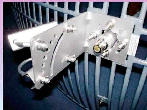
**Parabole TP-Link TL-ANT5830b : montage**
